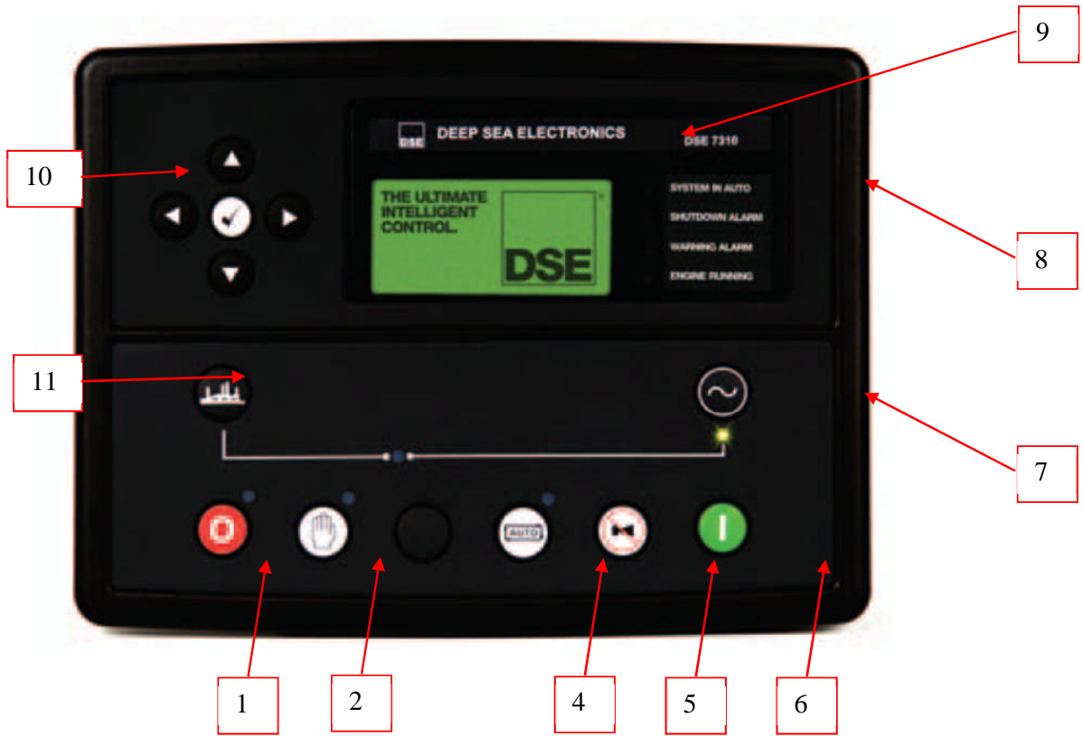
Picture 15- Deep Sea 7310 control module
